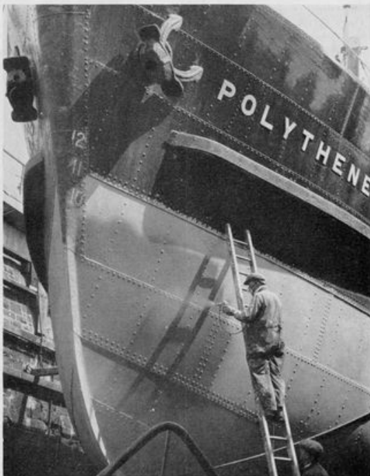
This picture shows the M.V. Polythene, an I.C.I. coasta. vessel, being coated with Evodyne thixotropic chlorinated rubber paint. (Report in the July issue of The Evodian)
