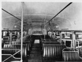
One of the new 'Fleetline' Omnibuses built by M. H. Cars Ltd., Dunsion, County Antrim, Northern Ireland. Ceiling of the lower deck and roof of the upper deck are lined with 'Darec' I.C.I. sheet, bonded with Evo-stik 'Impact' Adhesive 828. Photograph by kind permission of I.C.I. Plastics Division
